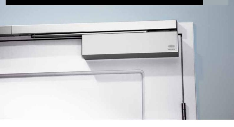
The Lockwood 2616EMC is a small single door electromechanical hold open device system with a sliding arm. It is applicable for places, where fire doors are constantly kept open. The door is kept open at a selected angle. If fire breaks out, the door is closed, preventing smoke and flames from spreading. Applications for 2616EMC include hotels, office buildings and other fire doors where hold open function is needed.
